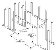
Figure 6 - Framing Dimensions Prior to Placing Appliance
